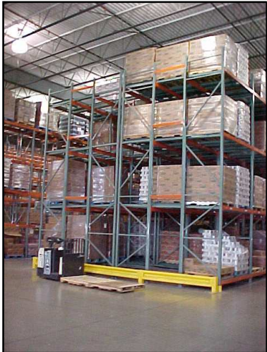
Push back rack system, 3 deep by 4 high, Interlake
