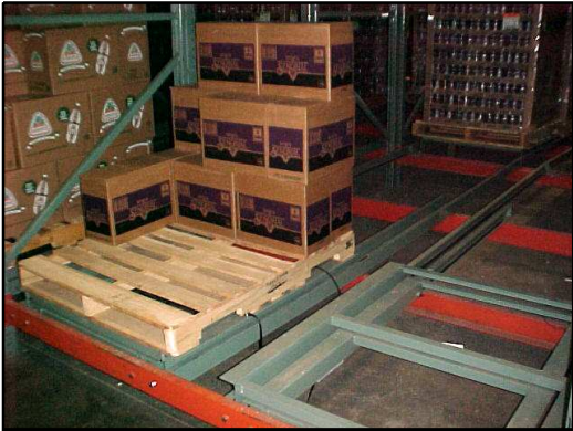
Push back rack system, 3 deep by 4 high, Interlake
