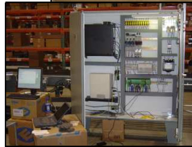
View of scale, scanner, control Cabinet and NBS-30 sorter running at 200 FPM.
