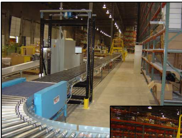
View of scale, scanner, control Cabinet and NBS-30 sorter running at 200 FPM.
