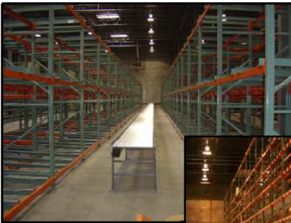
Carton flow rack in a single level pick module
