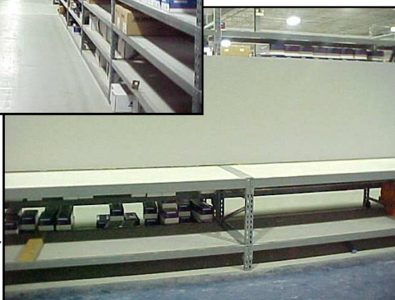
View of the typical work bench with integrated lower shelf and "backstop" riser.
