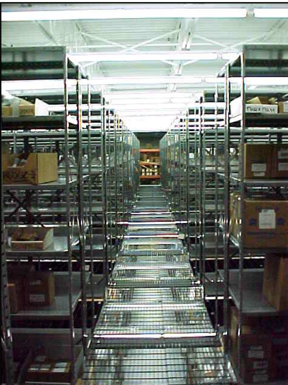
View of the upper level of the two-tier shelving system showing bar grate cat-walk system.
