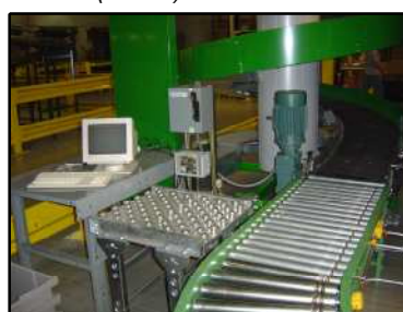
Outside view of pick module (above), tote induct station for orders (below)
