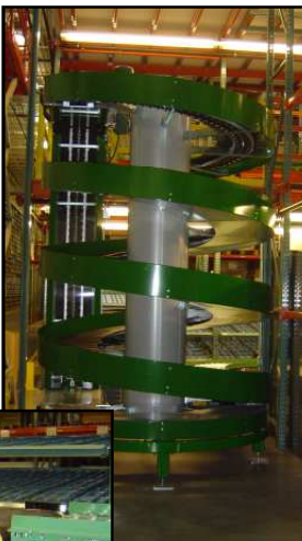
Main overhead line (above), spiral incline conveyor (right), conveyor-top scale for checkweighing orders (below)
