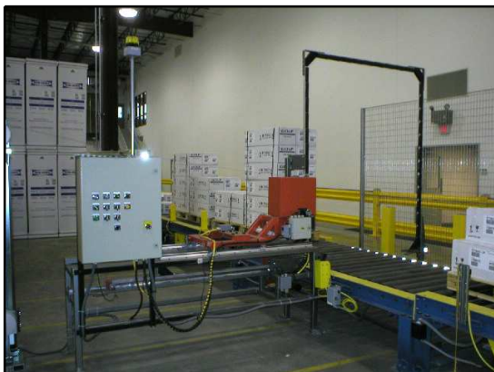
View of automated strapper with it's own control cabinet (left) and partially-completed control cabinet for conveyor (above).
