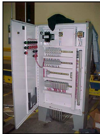
View of automated strapper with it's own control cabinet (left) and partially-completed control cabinet for conveyor (above).
