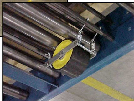
View of centrifugal brake (from underneath) that controls speed of pallet flow.
